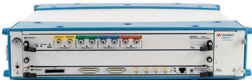
The M8195A arbitrary waveform generator packs as many as four differential channels with 65 GSamples/s sampling rate and 20-GHz bandwidth into a single AXIe module.
