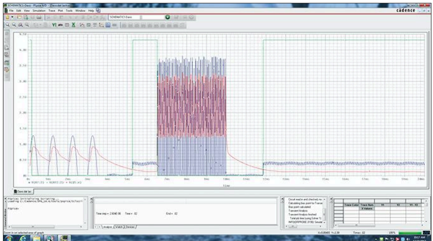
3. The noise bursts are set at 1.25 and 3.5 V, and the contact resistance is 0.4 \Omega , indicating a resistance of 20 \Omega .
