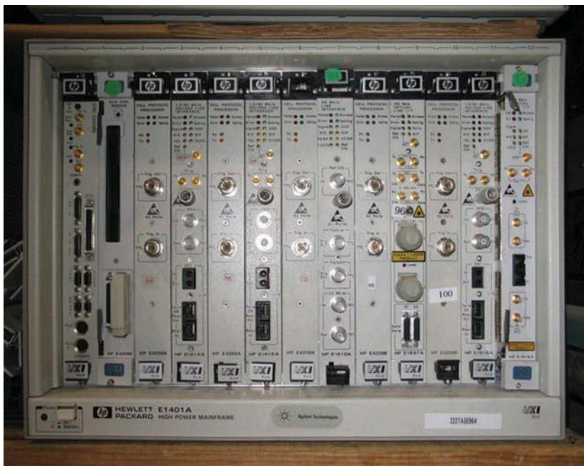
1. This VXI chassis illustrates the close spacing of modules and small instrument size possible even when realizing multiple measurement functions. [Photo courtesy of Alimar Technology ( www.alimartech.com ).]
